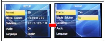
Format your SD car. After SD card fromat completed, press "A" key to back to Non-recording mode and press "F" key to start record the video
